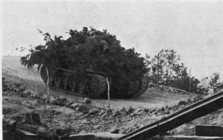
Only its running gear identifies this M-4 tank. It has three pairs of tandem bogie wheels like the M-7 (below) and the M-10 (top).
